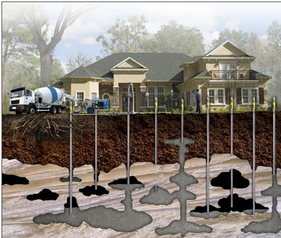
Subsurface Grouting courtesy of: http://www.foundationsservicescf.com/uploads/images/sinkhole-lb-large.jpg
