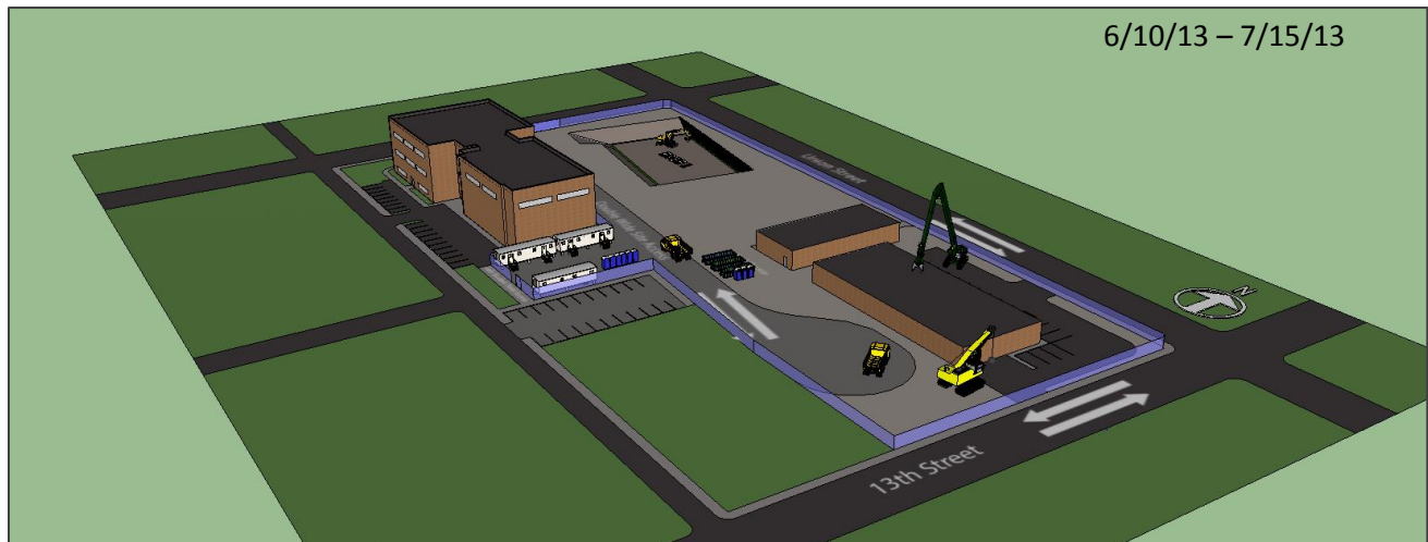
Figure 11: Demolition logistics plan.
